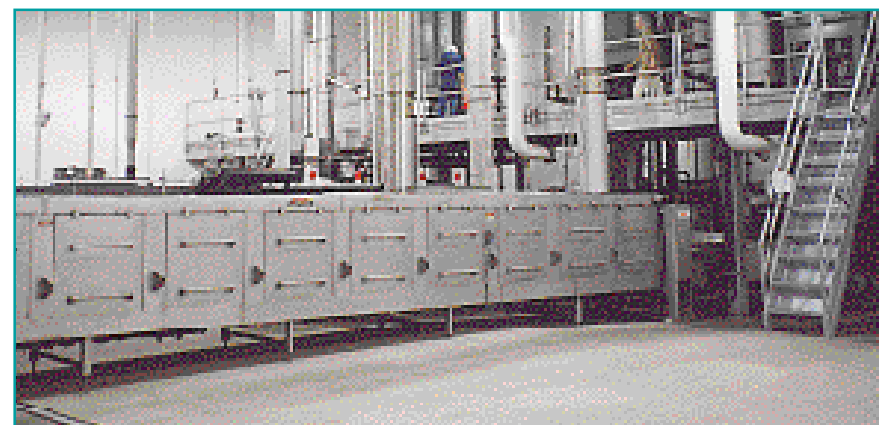
Single-Pass Toaster Ovens are available for tortillas, taco shells and other baked products.
